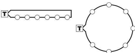
3. Split load installation or multiple cable run: Fixtures run in two or more directions from
